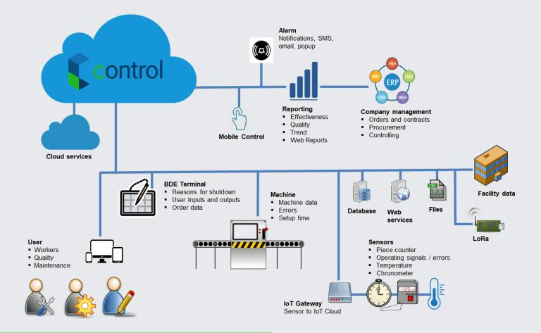
The monitoring solution **control** creates transparency, optimizes process management and enables automated workflows.
